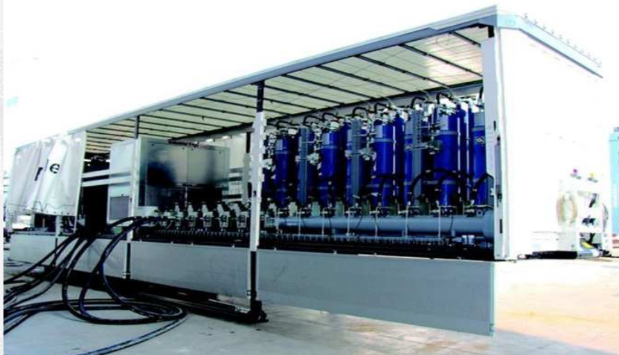
Mobile Laboratory for hydraulic power supply up to 6.000 l/min, 350 bar
