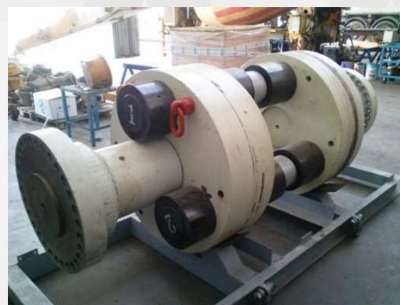
Calibration System for components up to 25 MN
