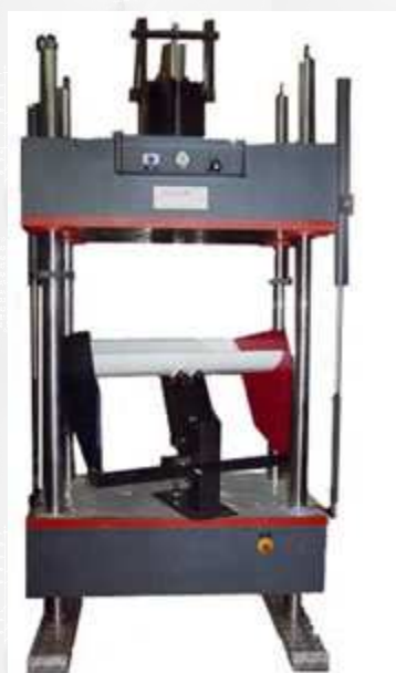
Load frame for Automotive: 500 kN load 2.000 mm. stroke
