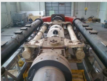
Biaxial System for Traction (25 MN) and Bending (1 MN/m) Tests
