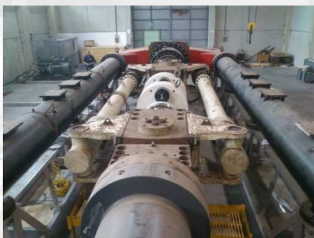
Biaxial System for Traction (25 MN) and Bending (1 MN/m) Tests
