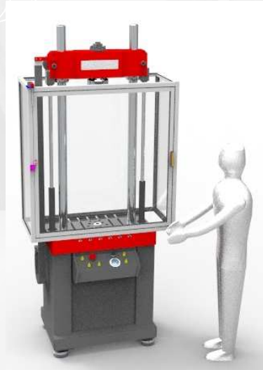
Servohydraulic Monoaxial 100 kN Machine
