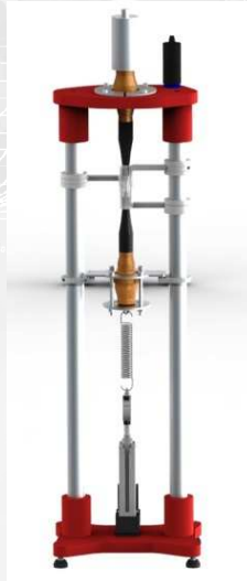
VHCF Machine for Fatigue test
