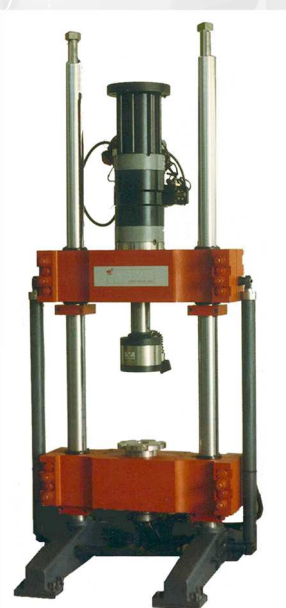
Load frame with 2 columns with light up to 3.000 mm.
