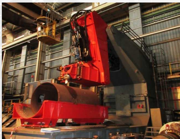
Damage Tests System on "Full Scale" piping
