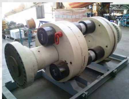
Calibration System for components up to 25 MN
