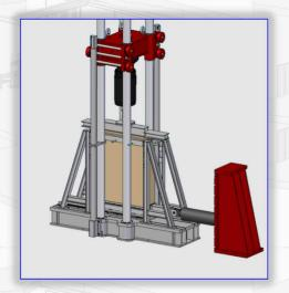
The maximum vertical load is 500 KN.
