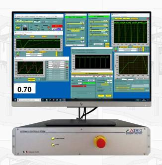
The RT3 control system is managed by an application software that works with a Real-Time operating system (working in deterministic mode without the inconvenient of the latency times caused by Windows environment) and is interfaced by an Ethernet link with a normal PC in a Windows environment, where reside application software developed with LabVIEW for the system management, the user interface, the configurations database, the data acquisition and operator front-end.
