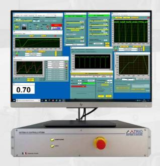
The RT3 control system is managed by an application software that works with a Real-Time operating system (working in deterministic mode without the inconvenient of the latency times caused by Windows environment) and is interfaced by an Ethernet link with a normal PC in a Windows environment, where reside application software developed with LabVIEW for the system management, the user interface, the configurations database, the data acquisition and operator front-end.
